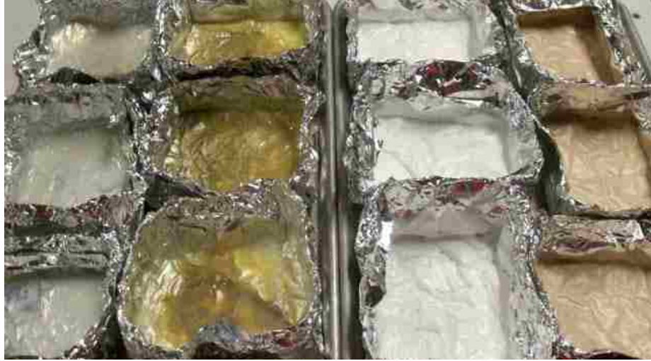
Figure 5 – Solid content of WLP and SBR samples (from left to right SBR1, SBR2, WLP1, and WLP2)
