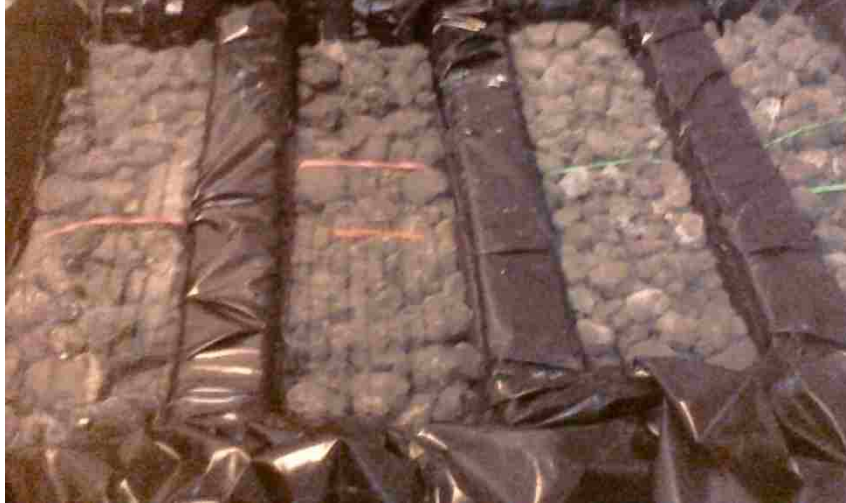
Figure 19 – Pervious concrete in freeze-thaw test
