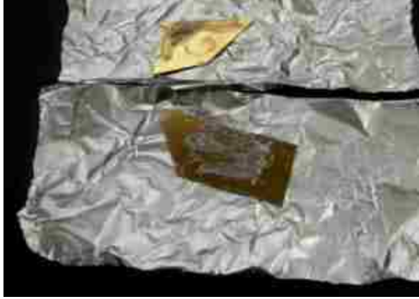
(c) Phase 2 – Dried paint on gold substrate
