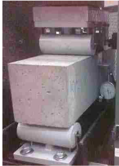
Figure 13 – Flexural strength setup
