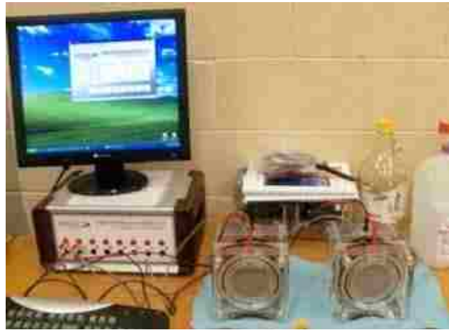
Figure 16 – Rapid chloride penetrability test setup
